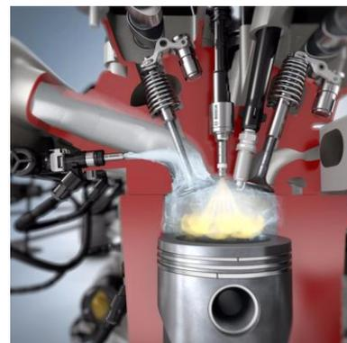
Figure 13 Bosch Waterboost System
